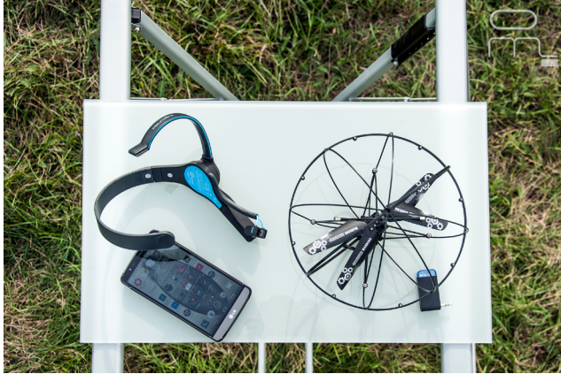
Il. 3 Mobile EEG device used during the first test of the experiment _e.1/2015–2017 , Mind Wave Mobile, Puzzle Box Orbit . Photographer: Viola Kuś. © Art & Science Research Foundation om – organisms and machines in culture . Bydgoszcz, Poland.
